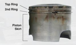
The piston rings earned a perfect merit rating of 10, demonstrating no-stick performance. The piston skirts demonstrated 0.00% scuffing, proving HP Marine's superior lubricity and friction-reduction capabilities.
