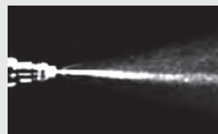
Injector spray pattern before P.i. treatment.
