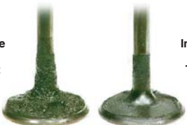
Intake Valve before P.i. Treatment
